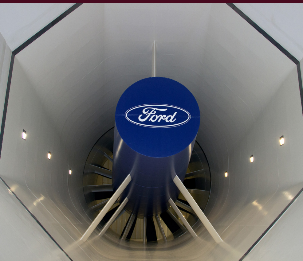
The wind tunnel fan blows air up to 200 mph and includes a state-of-the-art rolling road system.
